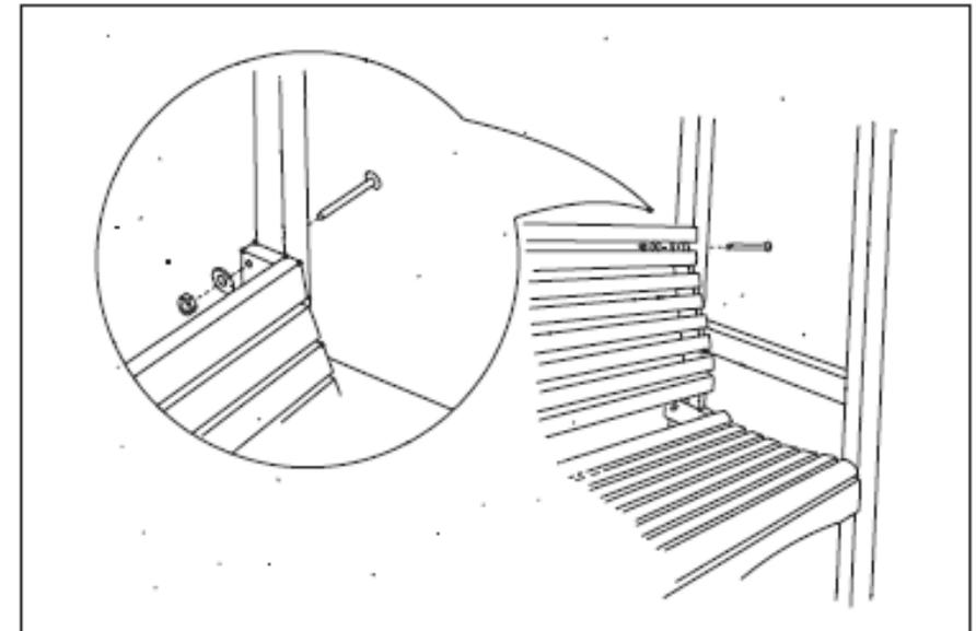
Carefully stand the seat and sides upright - this is best done by two people. Locate the back-rest into position and coach-bolt into place through the rear uprights.
