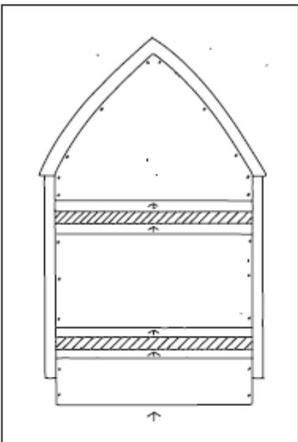
Finally, locate the back panels into the grooves in the cross-members as shown. Start at the top and screw into place as you progress down. Use 18mm flat head screw.
