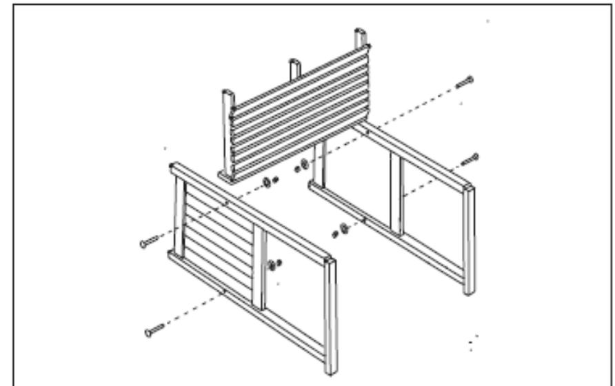
Now place the sides on the ground in the position shown. Lower the seat base into its location with the front edge of the seat on the ground. Secure in place with a coach-bolt at each corner.
