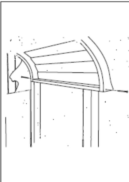
Lift the roof assembly into place and screw to uprights at each corner using the 60mm screws. Please do not overtighten screws.
